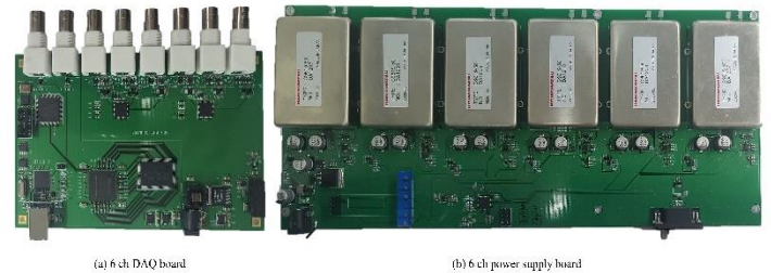
Fig 8. (a) The DAQ system and (b) the high voltage power supply board
