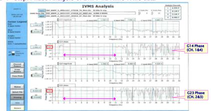
■ 1st Step Result: Fig. 2 shows the IVMS data which present the 180° phase shifts of signals from the middle (MD) detectors in ENFMS CH.1&4(G14) and from the lower (LW) detectors of CH.2&3(G23) detectors in the freq. ranges of 2 to 11 Hz.
