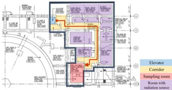
Fig. 2. Path and work space of sampling workers after LOCA
