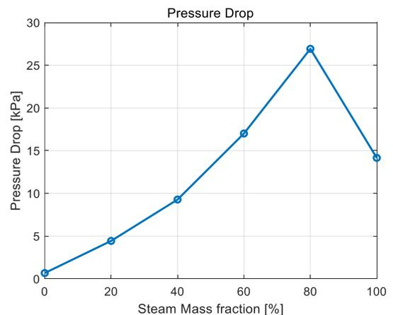
Fig. 6. Helical tube Pressure Drop by CFD calculation
