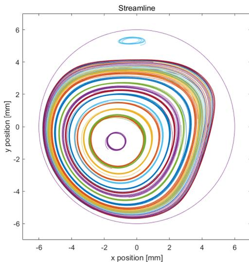
Fig. 13. Streamline (Mass fraction Steam 60%)
