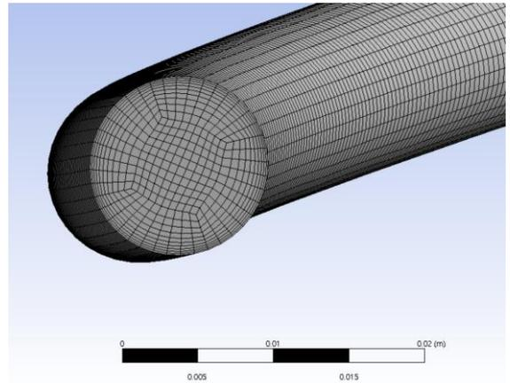
Fig. 5. Helical tube mesh for CFD analysis
