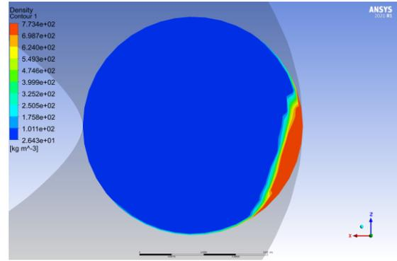
Fig. 9. Density Contour for a cross-section of a helical pipe (Mass fraction Steam 60%, Water 40%)
