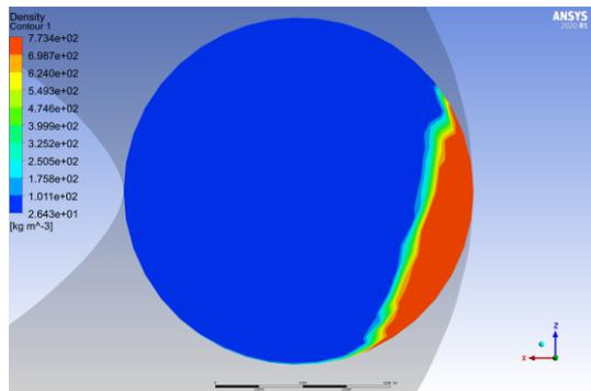
Fig. 8. Density Contour for a cross-section of a helical pipe (Mass fraction Steam 40%, Water 60%)
