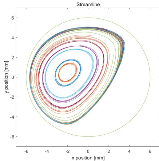
Fig. 11. Streamline (Mass fraction Steam 20%)
