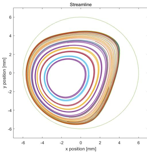
Fig. 12. Streamline (Mass fraction Steam 40%)
