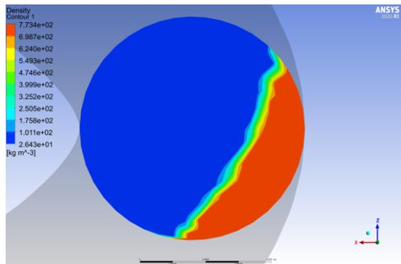
Fig. 7. Density Contour for a cross-section of a helical pipe (Mass fraction Steam 20%, Water 80%)
