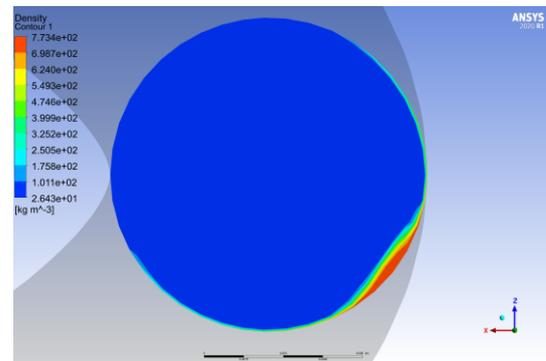
Fig. 10. Density Contour for a cross-section of a helical pipe (Mass fraction Steam 80%, Water 20%)
