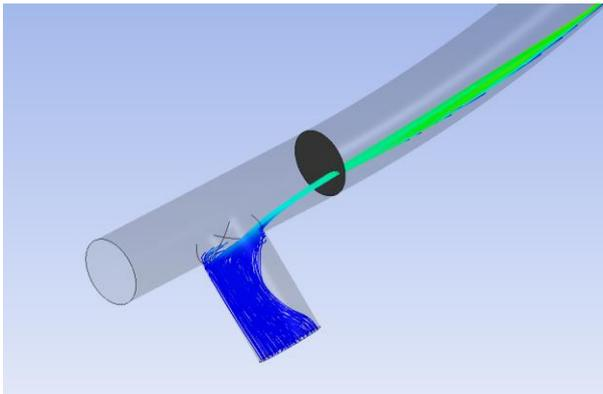
Fig. 3. Streamline of water near the inlet boundary (Mass fraction Steam 80%, Water 20%)
