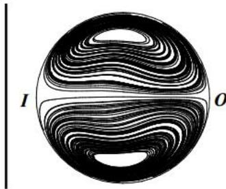
Fig. 1. Streamlines of the secondary flow in a helically-coiled tube [3]
