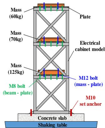
Fig. 1. Unit Under Tests(UUT)
