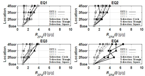
Fig. 4. Ratio of acceleration response spectrum
