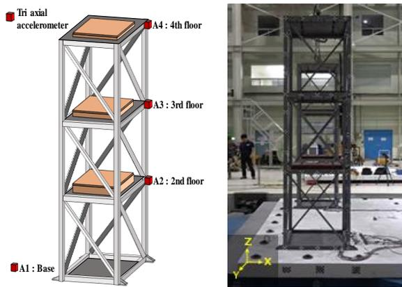
(a) Accelerometer location (b) Test photo
