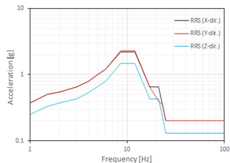
Fig. 2. Required response spectrum
