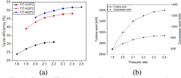
Fig. 4. Cycle efficiency according to the pressure ratio
