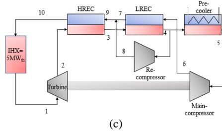
Fig. 1. Heat pipe cooled microreactor (a) Primary system [5] (b) Heat pipe (c) s-CO<sub>2</sub> recompression Brayton cycle
