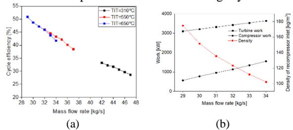
Fig. 3. Cycle efficiency according to the mass flow rate (a) Cycle efficiency (b) Works of turbine and compressor
