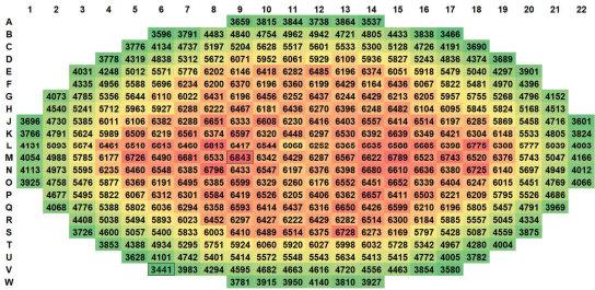
Fig. 3. CCP calculation result applying revised CHF correlation for the specific HSP-3 case A.
