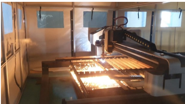
Fig. 4. A plasma torch cutter and an oxy-fuel cutter in Busan Machinery Research Center.
