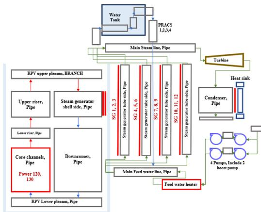
Fig. 2. MARS-LBE nodalization of MicroURANUS
