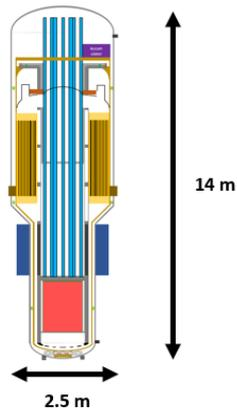
Fig. 1. Schematic diagram of MicroURANUS
