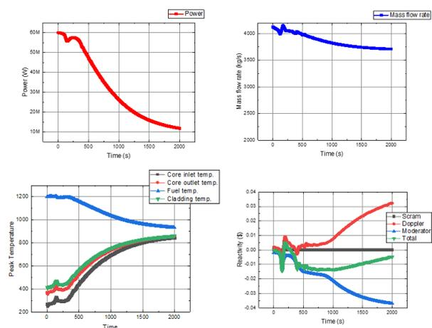
Fig. 4. ULOHS safety analysis result (Power, Mass flow rate, Temperature, Reactivity)
