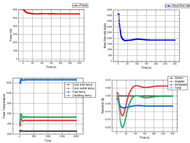
Fig. 3. ULOF safety analysis result (Power, Mass flow rate, Temperature, Reactivity)
