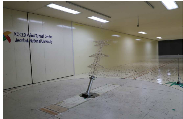
Fig. 2. Tilted model in the wind tunnel
