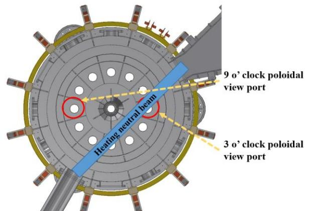
Fig. 1 position of the poloidal view ports for CES
