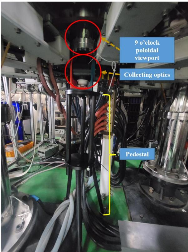
Fig. 2 Collecting optics at the 9 o'clock poloidal view port.
