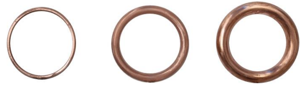
(a) d = 3 mm (a) d = 6 mm (a) d = 9 mm Fig. 3. Cathode rings for experiments.
