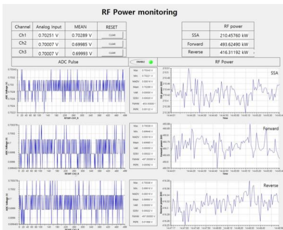
Fig. 4. Results of RF power output with respect to ADC input voltage (Enable state)
