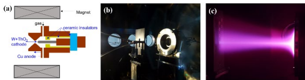
Fig 1. Description of KAERI divertor simulator: (a) schematic diagram of AF-MPD plasma source, (b) photograph of the KAERI divertor simulator, (c) operation of KAERI divertor simulator
