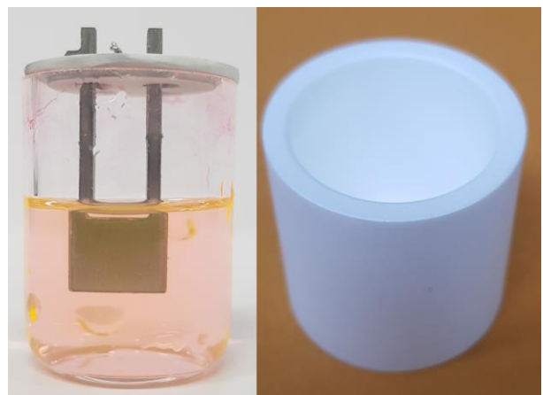
Figure 1. Structure of the corrosion cell with transparent Quartz (left) and BN crucible (right)
