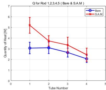
Figure 3. Bare, SAM tube heat transfer rate comparison
