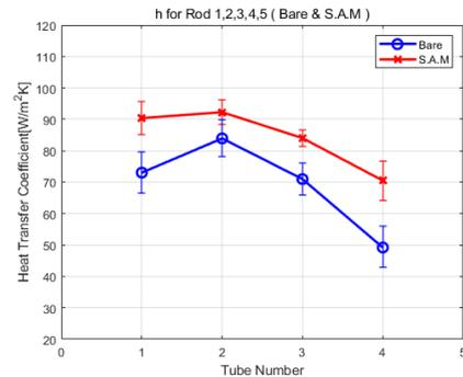
Figure 4. Bare, SAM tube heat transfer coefficient comparison
