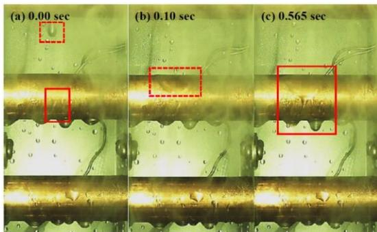
Figure 5. Droplet dynamic of flowing previous water path shown with bare copper tubes (tube 1 to tube 3)
