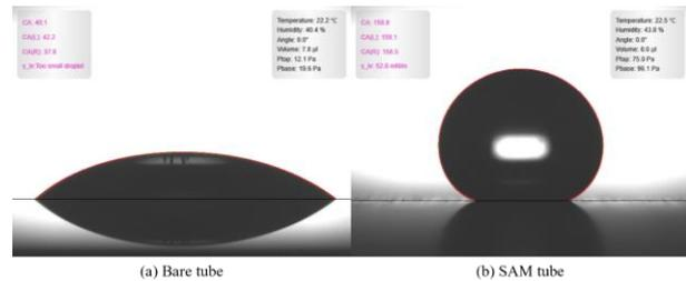
Fig. 1. Superhydrophobic surface modification result:
