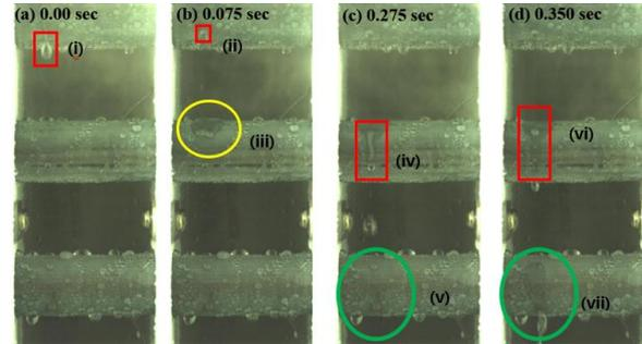
Figure 6. Droplet dynamics shown with superhydrophobic copper tubes (tube 2 to tube 4)
