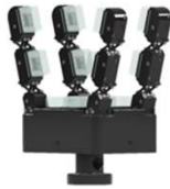
A type of hybrid gripper (presented by DGIST)
