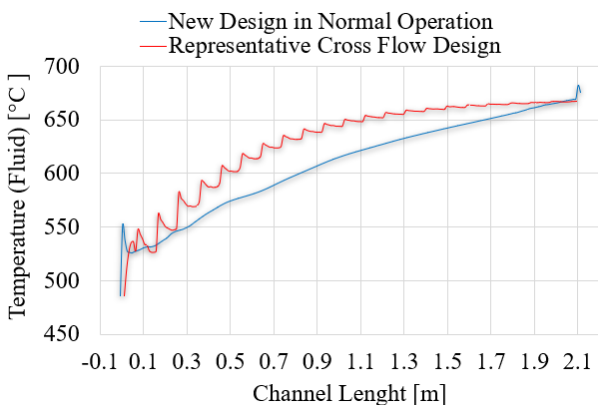
Fig. 6. Coolant temperature change through the channel length.
