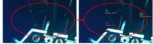
Fig. 4. Examples of qualitative air bubble detection on the HANARO reactor core. Columns from left to right correspond to original image and image with detected bubbles.
