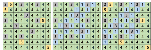
Fig. 2. Pin pattern of fuel assembly (bottom-right 1/4). Case1(left), case 2(center), case 3(right)
