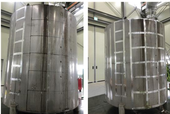
Fig. 3. Marking of the cutting area before the experiment(left) and sealing after cutting(right)
