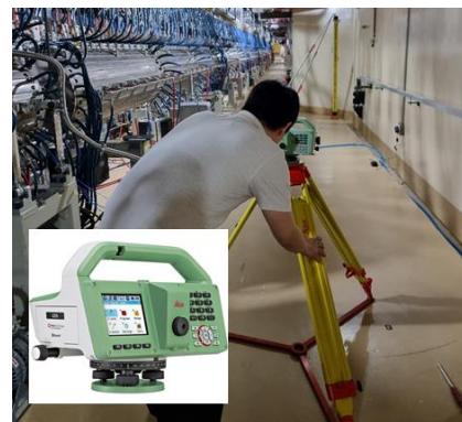
Fig. 6. Measurement of standard invar staff using the digital level (Leica, LS-15)
