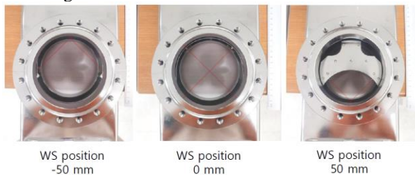
Fig. 1. Wire scanner (WS) is kept at -50 , 0 and 50 mm position and red lines are marked for better visibility of the wires.
