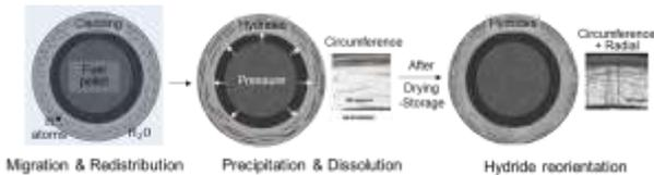
Fig. 1. Hydride rearrangement process of irradiated cladding
