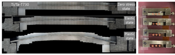
Fig. 2. Panoramic optical microscope (O.M.) photos taken before and after applying stress to the specimen using a jig, and the specimen was prepared with a TEM grid attached for further analysis..
