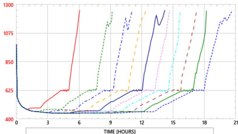
Fig. 3. Peak cladding temperature according to TD-AFW cooling time 1 h ~ 10 h [K]
