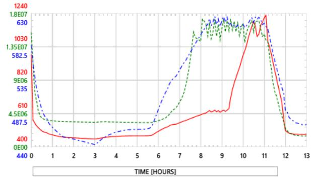
Fig. 4. Plant status of offsite power recovery (red: PCT [K], blue: core water temperature [K], green: PZR pressure [Pa])
