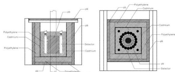
Fig. 1. Structure of He-3 proportional counter installed in HANARO DNAA system
