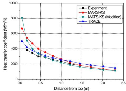
Fig. 5. Heat transfer coefficient for Exp. 3.4-3 (NC=20%)
