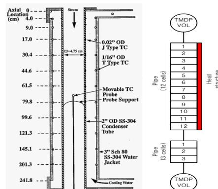
Fig. 1. UCB-Kuhn Test Section and Nodalization Diagram for MARS-KS code.
