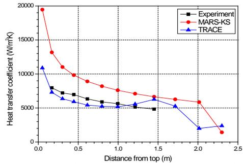
Fig. 4. Heat transfer coefficient for Exp. 1.1-1 (NC=0%)
