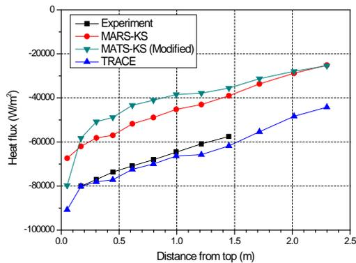
Fig. 3. Heat flux for Exp. 3.4-3 (NC=20%)
