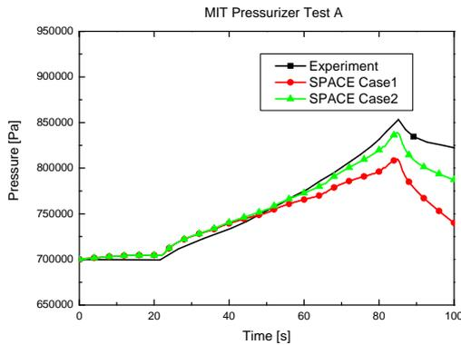
Fig. 2. Pressure vs. time for the MIT Pressurizer test : insurge into a partially filled pressurizer.
