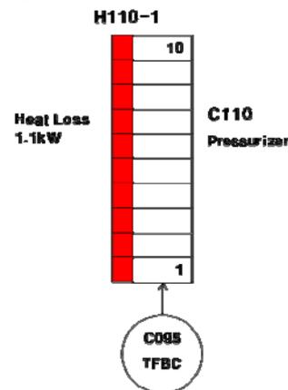
Fig. 1. SPACE Nodalization diagram for the MIT pressurizer.
