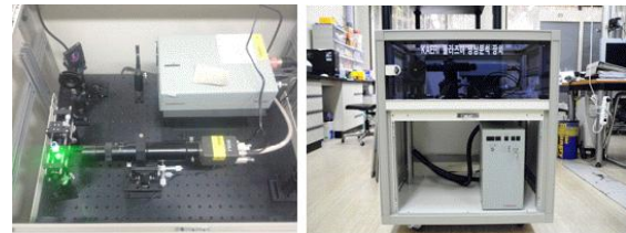
Fig. 1. A LIBD system used to determine the size and concentration of groundwater colloids.
