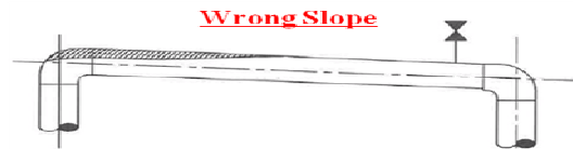
Fig. 3. Gas accumulation in pipe with wrong slope.
