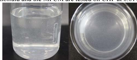
Fig 1. Dispersion status of MPCM in R-123 (0.01v%)
