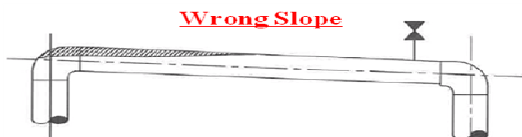
Fig. 1. Gas accumulation in pipe with wrong slope.
