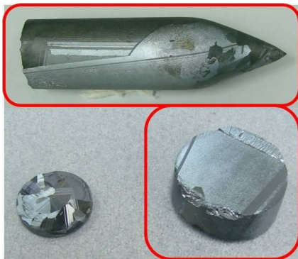
Fig. 1. The etched CZT ingot and the cut crystal, which were grown by 6-zone LP Bridgman furnace at KAERI.
