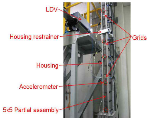
Fig. 1 Test Section of INFINIT Test Loop
