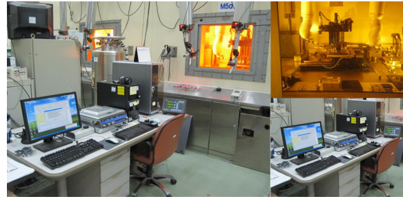
Fig. 5. After installation, (left) the picture of the whole system of the 3-D measurement apparatus, (top-right) a photo of in-cell parts, (bottom-right) a photo of out-cell parts.
