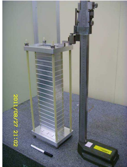
Fig. 8. Fabricated multi layer insulation DC break.
