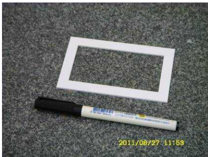
Fig. 6. Fabricated alumina insulator parts for DC break.
