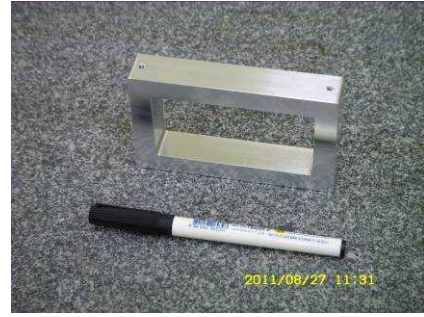
Fig. 7. Fabricated conductor parts for DC break.
