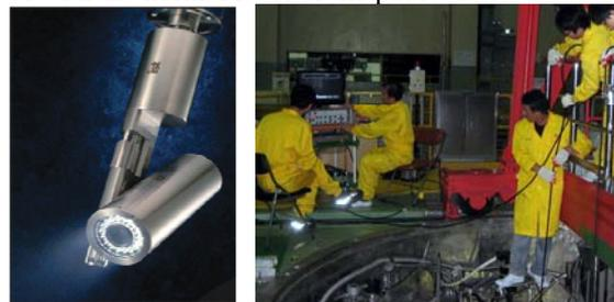
(a) Underwater camera (b) Camera controller and monitor
