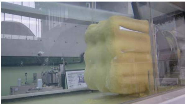
Fig. 3 Fiberglass debris accumulation at screen
