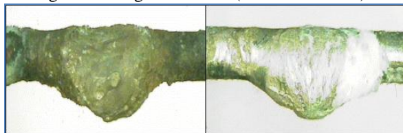
Fig. 3. Status after flaming heating without twist (Inconel/STS310)
