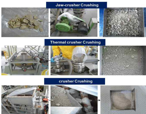
Fig 1. Uranium contaminated concrete crushing test
