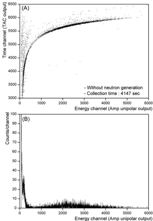
Fig. 3. Two-dimensional distribution of energy and time for background radiation (A) and the corresponding energy spectrum (B).
