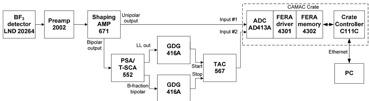
Fig. 1. Block diagram of the system for the discrimination of neutron and background pulses of the BF<sub>3</sub> detector.
