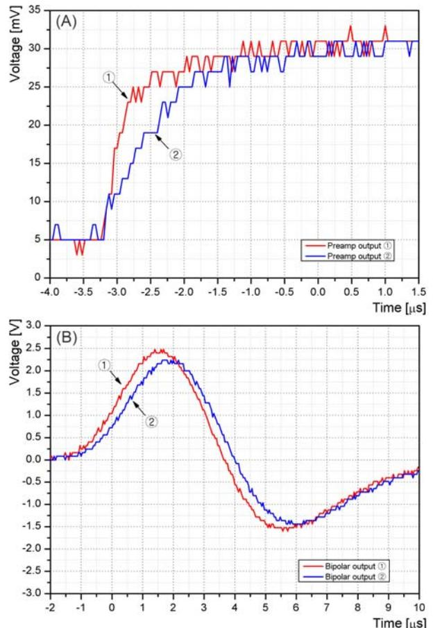
Fig. 2. Two preamp pulses with different rise time (A) and corresponding responses of the bipolar shaper (B).
