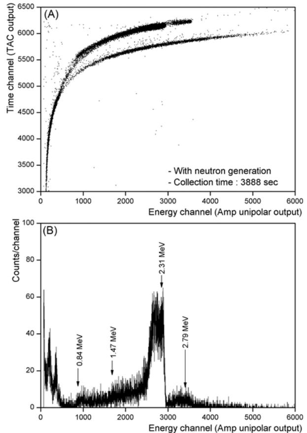
Fig. 4. Two-dimensional distribution of energy and time during the neutron generation (A) and the corresponding energy spectrum (B).
