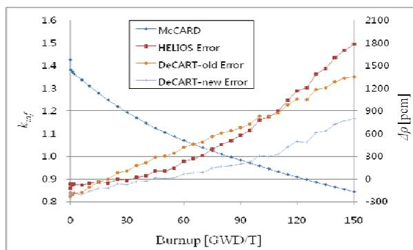
Figure 2. Depletion results for the PMR200 fuel cell
