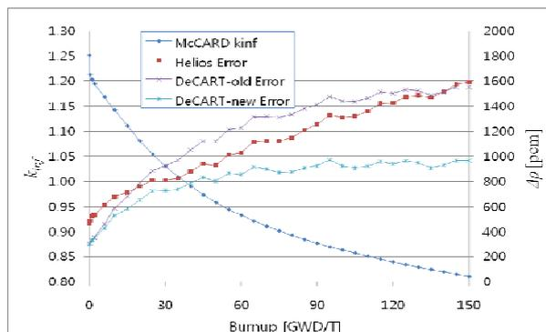
Figure 1. Depletion results for the homogeneous fuel
