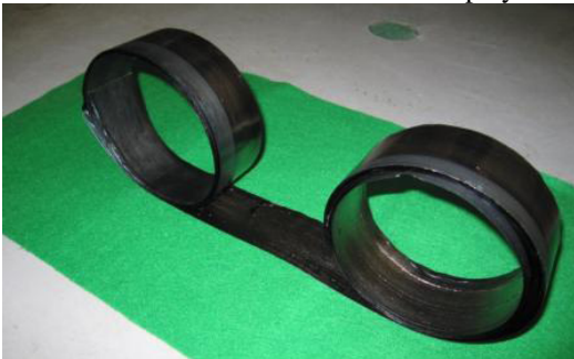
Fig. 2 U Foil produced by roll casting about 10meters
