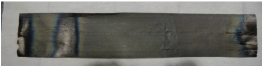
Fig. 3 U foil which Average thickness is 120\mu\text{m}
