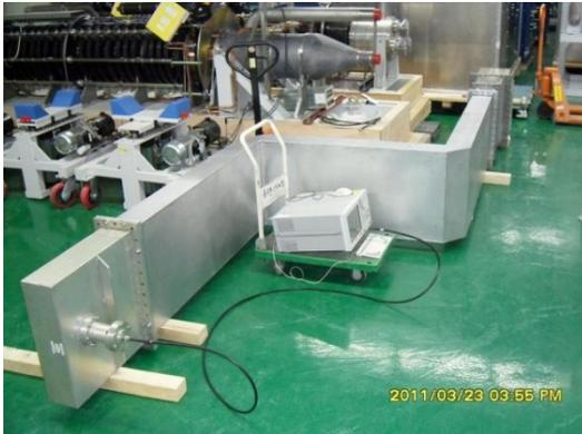
Fig. 5: VSWR measurement for the waveguide penetration section.
