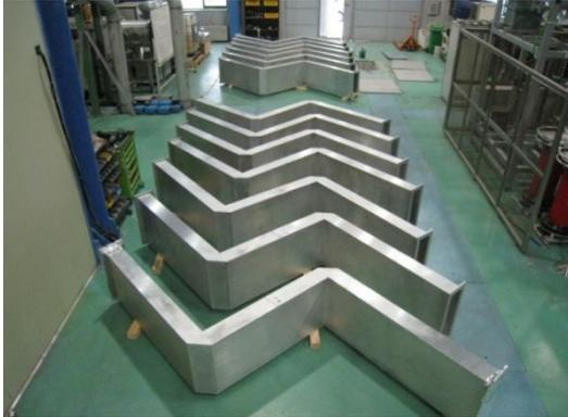
Fig. 4: Fabricated waveguide penetration sections
