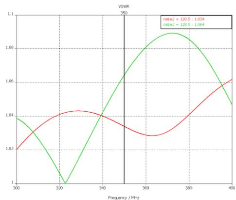
Fig. 3: VSWR calculation considering the chamfer error
