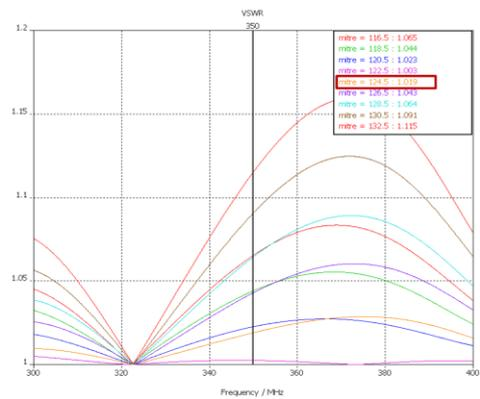
Fig. 2: VSWR calculation for the waveguide penetration
