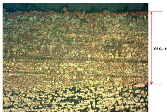
Fig. 3. Cross-sectional view of optical micrograph for C26000 brass, selectively leached for 50 hours in a 1% CuCl 2 aqueous solution at 75 C.
