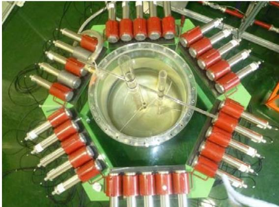
Fig. 2 Experimental apparatus of Industrial Single Photon Emission Tomography
