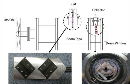
Fig. 4. Schematics of slit and collector system
