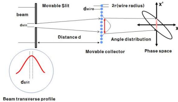
Fig. 1. Schematic of the slit and collector method for measurement of transverse beam emittance.
