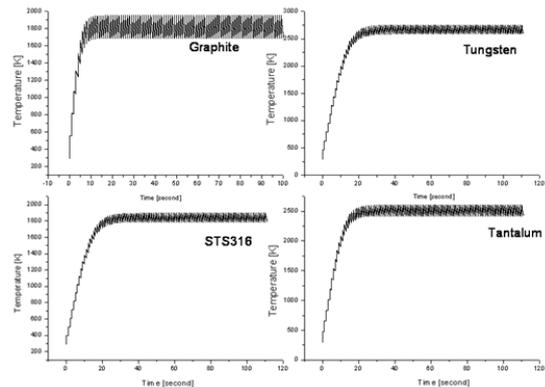
Fig. 3. Thermal load of materials for the slit under beam conditions
