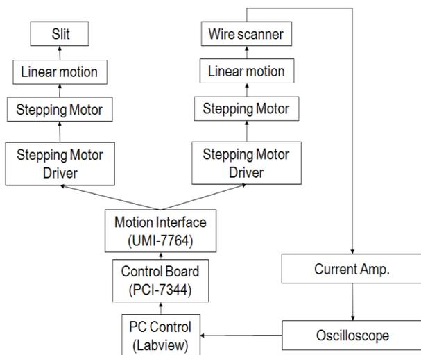
Fig. 5. Block diagram of the slit-collector system
