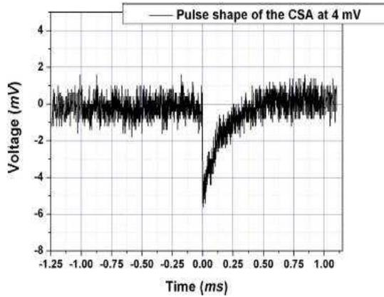
Fig.3. SP-110 Preamplifier Output signal
