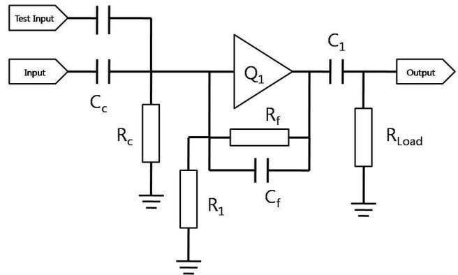
Fig.1. The schematic diagram of AD829A Preamplifier circuit. ( $C_c=100$  nF,  $R_c=1$  k $\Omega$ ,  $R_f=2.2$  k $\Omega$ ,  $C_f=60$  pF,  $R_1=300$   $\Omega$ ,  $C_1=4.7$  uF,  $R_{Load}=47$   $\Omega$ )
