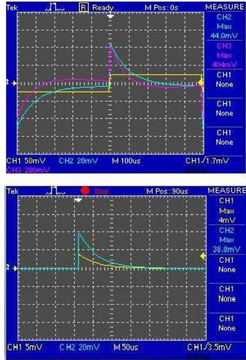
Fig.4. Pulse shape of AD829A(upper) and AD8510 (lower) output signal
