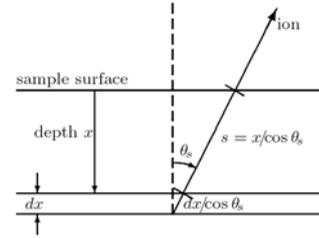
Fig. 2. Path of charged particle born at depth  $x$  that reaches the NDP detector.
