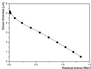
Fig. 3. Path length in silicon versus the mean residual energy.
